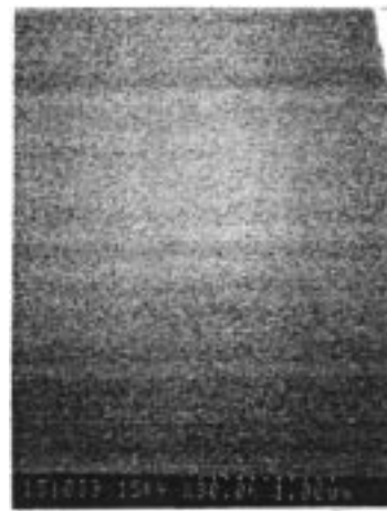
Fig. 3. SEM of the surface of a sputter deposited ZrO 2 film exhibiting a featureless surface structure.
